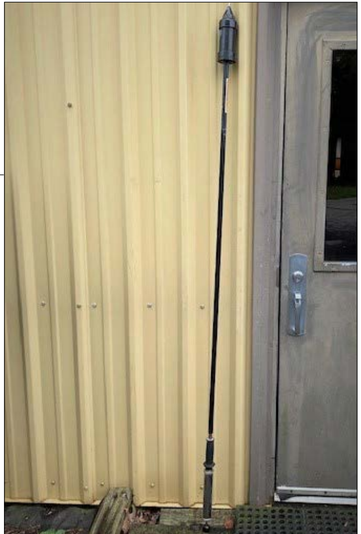
(Bottom) Long pole insecticide duster (Dustick) can help apply dusts to high nest location and at a safer distance for the applicator. Photo credit: Eric Benson, Clemson University.
